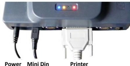
The other end of the **Mini Din** is connected to the **iPigeon Clock**
