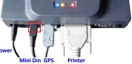
The other end of the **Min Din** is connected to the **iPigeon Clock**
